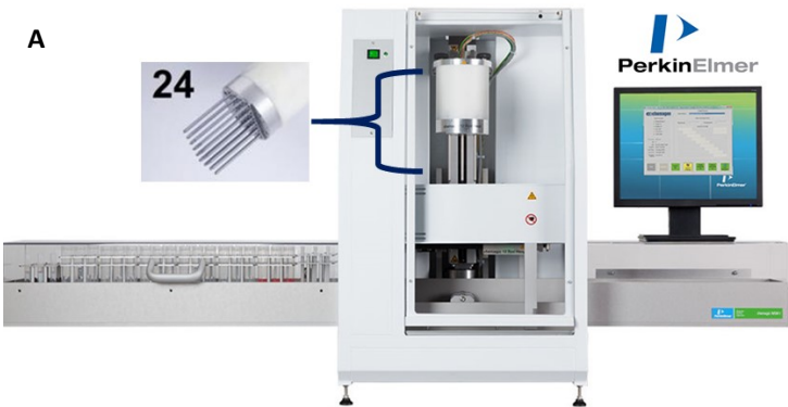
Figure 2. (A) PerkinElmer chemagic MSM I instrument with a close up image of the chemagic 24 Rod Head. (B) DeckLayout for the Processing of the iSWAB-DNA Samples on the chemagic MSM I.
