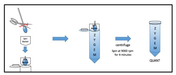
Figure 3. Visual Representation of Sample Preparation for ZyGEM Reaction
